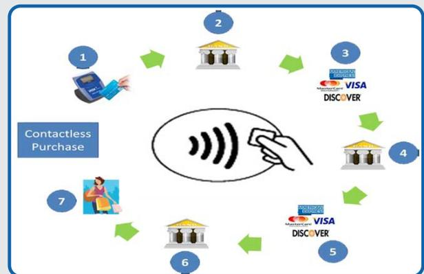
1. The cardholder passes the contactless card close to the contactless card-reader POS device within the range of approximately 2 - 4 inches from the device. The card-reader captures the data encoded on the contactless card.
